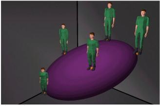
Figure 4. Illustration depicting the concept of boundary manikin human figure model
